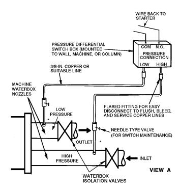
Fig. 14 — Typical Nozzle Piping
